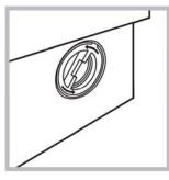
2. 以逆時針方向擰開過濾器 溫馨提示:打開時通常會有少量餘 水溢出,屬正常現象;可先在過濾 器前方放置吸水物料或毛巾 unscrew the lid by rotating it anti clockwise: a little water may trickle out. This is perfectly normal
