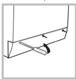
1. 以螺絲批鬆開機前部擋板(見圖) using a screwdriver, remove the cover panel on the lower front part of the washing machine (see figure)
