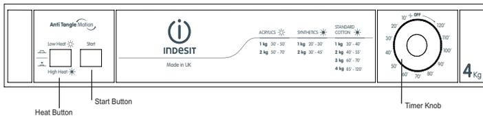
The HEAT button selects drying temperature.
