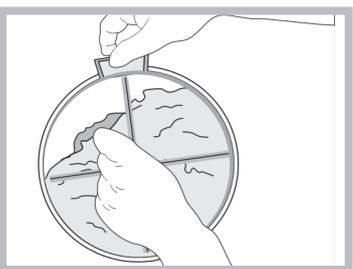
**Step 3** - Make sure the filter is pushed fully home - **NEVER** run the dryer without the filter in position.
